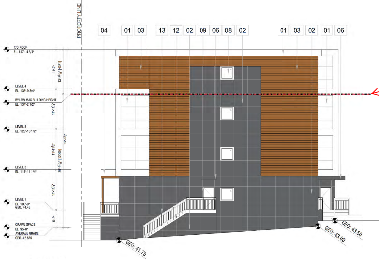
1 NORTH ELEVATION DP3.1 SCALE: 3/16" = 1'-0"
